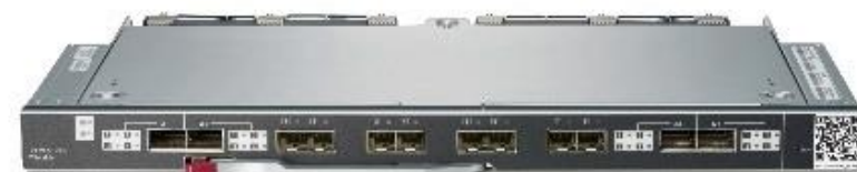
Brocade 16Gbit SAN Switch
